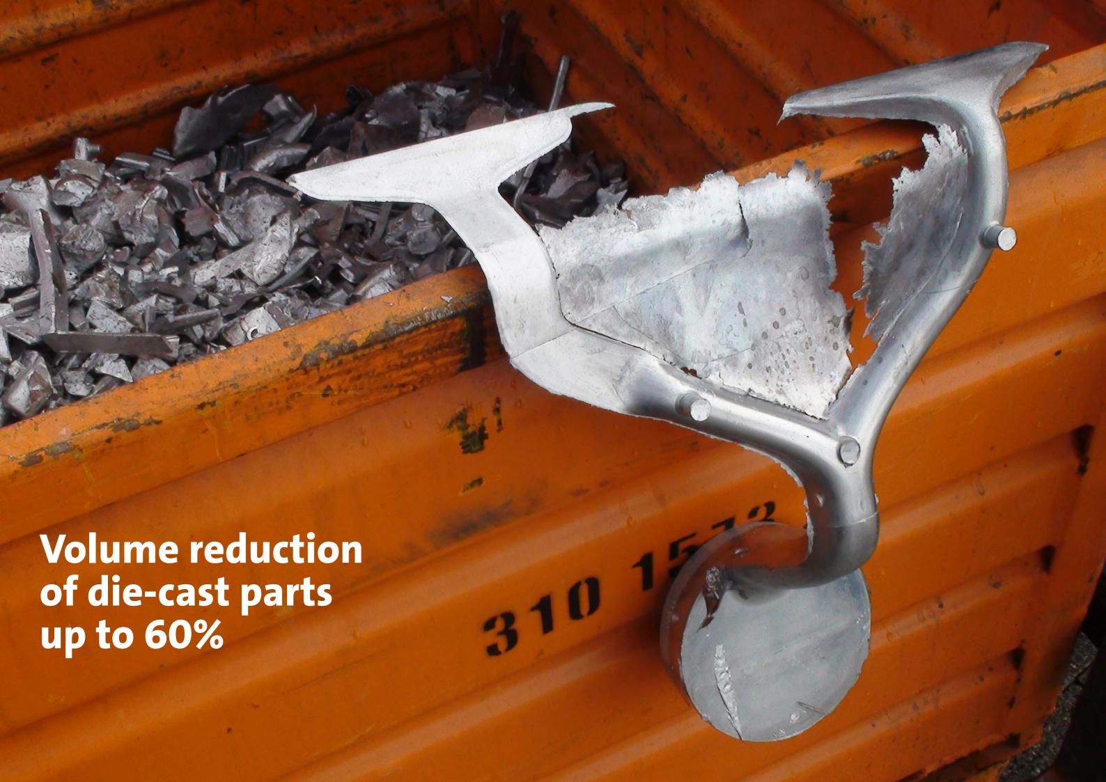
The scrap parts fall directly from the press into the hopper of the shredding plant and then into containers. These are regularly emptied into a large container and then transported to the smelter.
