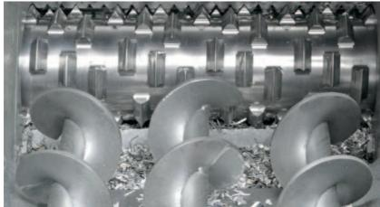
3-SCREW-SWARF-SHREDDER. RECYCLING AT ITS BEST.
